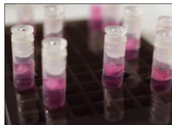
Codes can be verified either prior to or after thaw. If the database is used properly, the user avoids problems with condensation or frosting during the reading process, as the tubes can thaw prior to checking the codes. Condensation and frost are problems that can be overcome by wiping the codes, having them covered during storage or using dehumidified air.
