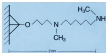
Schematic chemical and physical configuration of the CovaLink NH surface. The NH groups are spaced from the polystyrene surface by approx. 2 nm long, chemically defined spacer arms, and are covalently anchored to the surface.
