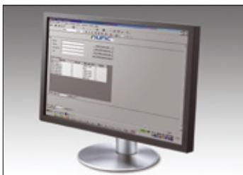
The database program uses the location of the vials in the rack, the location of the rack in the freezer, and the associated sample data to keep track of the position of every sample and combine it with the data used for selecting samples at retrieval.
