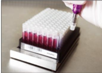
Removal of caps can be easily automated using a socket that snaps into the cap. Our partners offer 96 head decappers using this technique.
