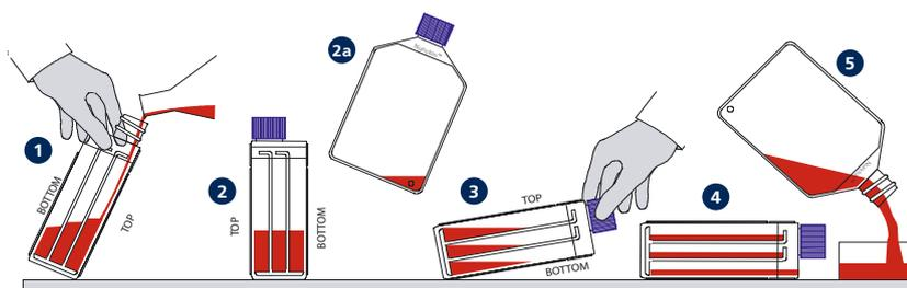
1. Prepare homogeneous cell suspension. Pour into the TripleFlask, tilting flask slightly to avoid foam or bubbles. Recommended working volume is 100-200 ml
