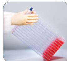
4. With filling inlet up, carefully tilt the CF EasyFill™ to a horizontal incubation position. Handle by holding on to the sides - do not manipulate by holding on to the upper rim.
