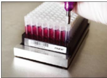
Caps are replaced using the single or multiple head screwdrivers. Vials are locked into the rack, which ensures that they do not fall out during transport in the lab or storage. The snap in the rack also retains the vial in the rack when the cap is mounted and the screwdriver is removed.
