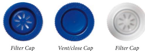
The caps for Nunc flasks are made of High Density Polyethylene (HDPE). This material is slightly flexible which means that a tight seal can be achieved without high torque. The caps should be turned by gripping the closed end as squeezing the open end makes removal more difficult.
