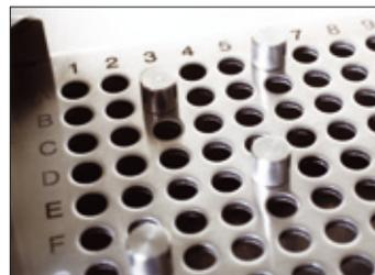
The racks are selected in the database program. Each rack can contain more vials than are required to be picked. The Nunc tube selection tool is intended for picking several vials out of a rack. While still at room temperature, the bits are placed in the positions listed in the database selection list. After verifying the bit position, the rack is ready to be taken out of the cold.
