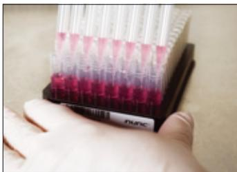
The cryobank vials are arrayed in a microwell format that allows for the use of multi-channel pipettors or liquid handling robots. This facilitates sterile work and minimizes handling time.
