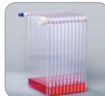
3. Turn the CF EasyFill™ 90°, so that the filling inlet is up. Media will be separated with equal amounts in each chamber.
