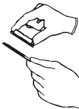
Gasket removal. Insert tip of a thin bladed spatula or similar tool under gasket at one corner. Without stretching or tearing the gasket, smoothly lift it away from the slide
