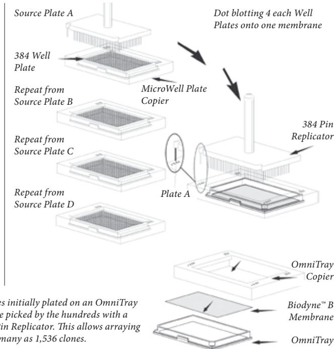
Clones initially plated on an OmniTray can be picked by the hundreds with a 384 Pin Replicator. This allows arraying of as many as 1,536 clones.
