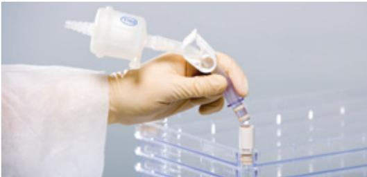
*PLUG* a media container into our standard port via a standard cell factory connector. Provides a semi-closed system for GMP production.
