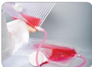
Fill or empty through the plug and play connection, and work with a semi-closed system.
