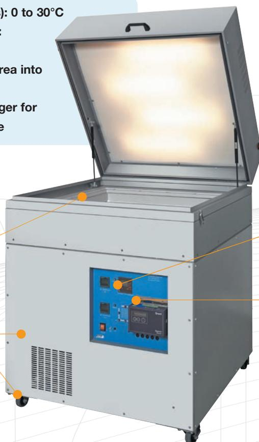
GRD1 temperature gradient plate shown with optional lid and integrated Squirrel data logger
