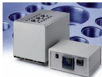
Block heater for oil testing
