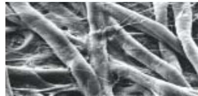
Whatman cellulose filter papers exhibit particle retention levels down to 2.5 \mu\text{m} .
