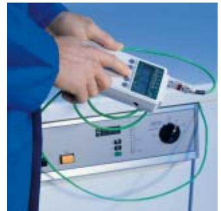
Access point for measuring temperature holding times
