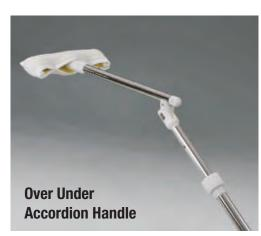
An electropolished stainless steel collapsible handle designed to deal with the unique space limitations in isolators and containment hoods. Available in 13" and 19" sizes, each section features a delrin hinge and quick disconnect to allow for attachment of additional sections and ultimately the mop adapter.
