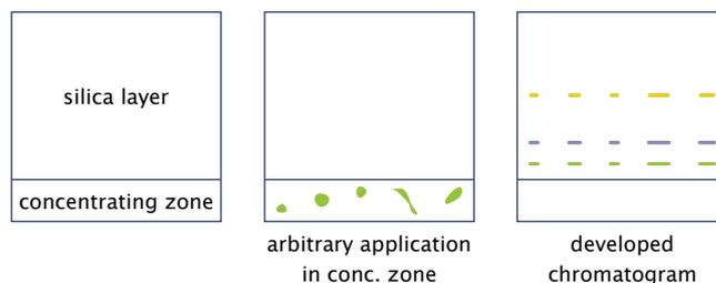
Another method for sample concentration is a short pre-elution (few mm) with a solvent, in which all substances have a high  $R_f$  value.
