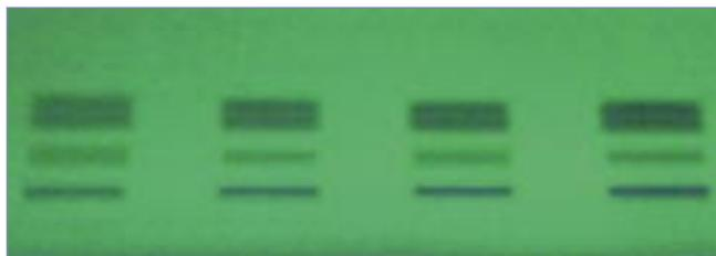
Identification of separated substances is possible via the  $R_f$  value compared to the pure compound, which is often applied simultaneously on the same plate.
