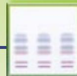
If a quantitative evaluation with a TLC scanner is to follow the separation we recommend to use commercially available sample applicators for spotting. These range from simple spotting guides via nanoapplicators to completely automated spotting devices. Application as streak can be performed automatically by spraying of the sample without touching the layer of the TLC plate. Application as band over the whole width of the TLC plate is especially important for preparative TLC.
